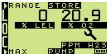
Fig. 4-10 H2S Sensor Fault
